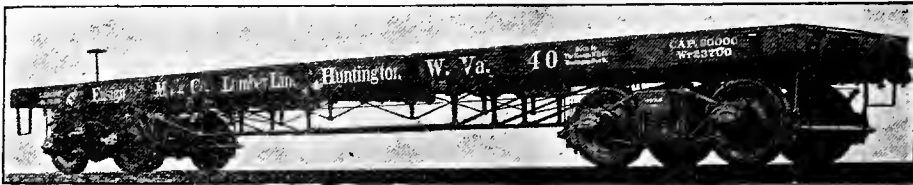
Fig. 19. FLAT CAR, FOR BRIDGE TIMBERS. Length, 41 ft. Capacity, 60,000 lbs. Weight, 23,700 lbs. Equipped with Rigid Diamond Trucks (Details are shown in Figs. 294-297.)
